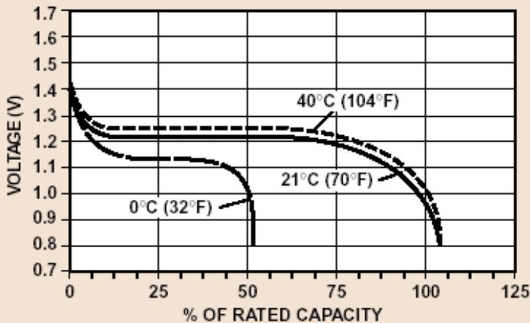
A zinc air battery discharged at the 75 hour rate at 0°C (32°F), 21°C (70°F), and 40°C (104°F).
