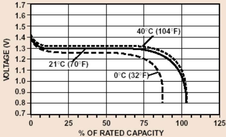
A DURACELL<sup>®</sup> zinc air battery discharged at the 300 hour rate at 0°C (32°F), 21°C (70°F), and 40°C (104°F).
