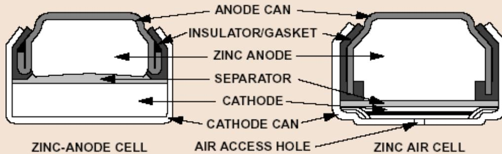
Cross sections of a typical zinc-anode cell and a DURACELL® zinc air cell are shown for comparison. The increased amount of anode material in the zinc air cell enables the cell to deliver greater capacity and energy density.
