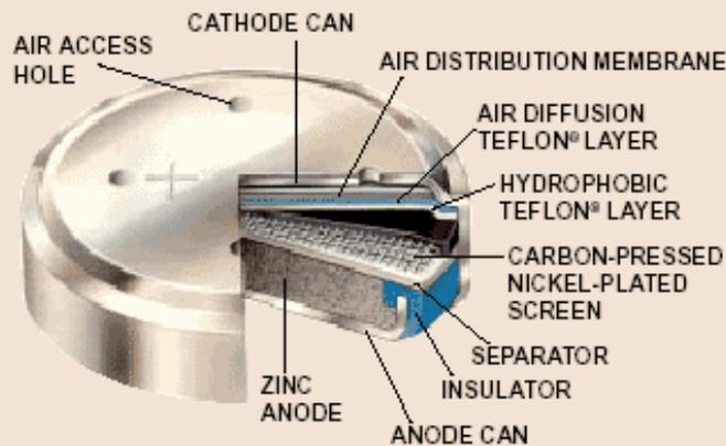
A typical DURACELL® zinc air cell is shown with the major components labeled for reference. (Note: The cell components are not drawn to scale.)
