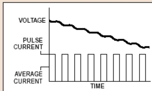
The voltage profile of a zinc air cell declines when the amount of air needed to support the average current drain is more than what can be supplied to the cell.
