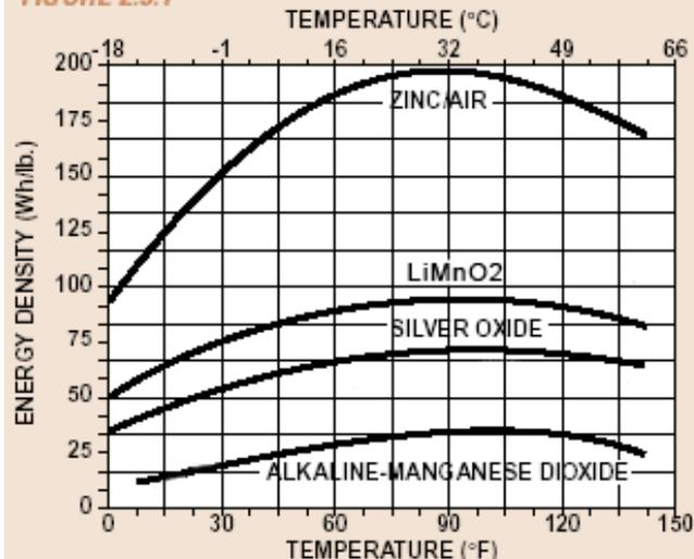
A comparison of gravimetric energy densities of primary button cells on a watt-hour-per-weight basis.
