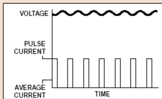
The voltage profile of a zinc air cell remains constant when the average current drain is able to be supported by the amount of air available.
